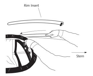
Slide into pocket on underside of coaming rim.
