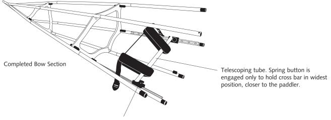
Thumb screws secure brace in position.
