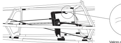
• Red webbing straps from rudder cable attaches to buckle on foot pedal.
