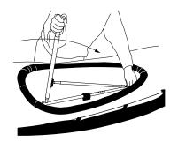
b. Insert Chine and Gunwale extension bars, keeping them in the sleeves of the seat sling. Double bands of tape indicate stern end.
